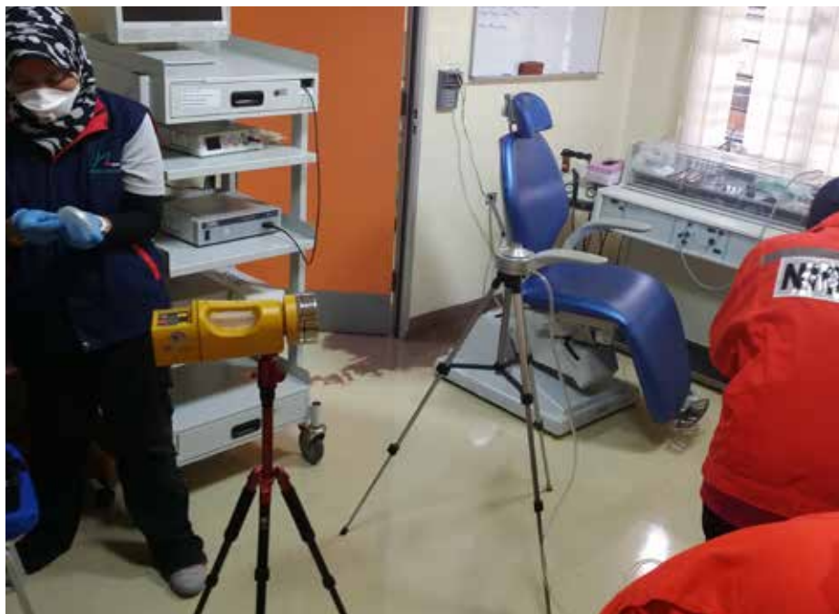
The IAQ level in Melaka Hospital (chosen as piloted site as a PSDT project) has improved with bacteria, fungus and volatile organic compounds having been eliminated after the spraying of TiO 2 nano solution
